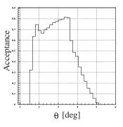
Figure 4.20: Detector acceptance of the SSD as a function of the angle in the laboratory flame. This data is obtained from the Monte Carlo simulation and Only the detector geometry is considered in the simulation.
