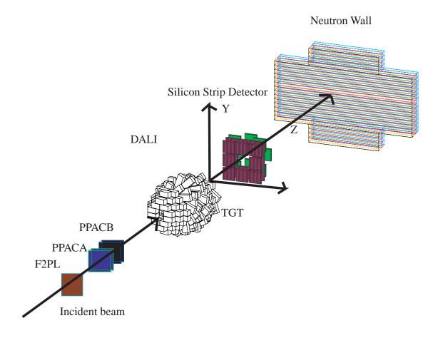
Figure 3.3: Schematic view of the setup backward F3. The detectors system comprises 152 NAI(Tl) detectors for detecting  $\gamma$ -rays,  $\Delta E - E$  Silicon Strip Detector for detecting outgoing reaction products, and Neutron Wall for detecting neutrons produced in the reaction.
