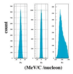
Figure 4.11: momentum vector of the incident beam. Momentum information was obtained by F2PL.
