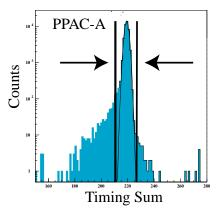
Figure 4.8: Spectra of the sum of timing  $(T_1+T_2)$  of both electrodes attached to a PPAC. Single hit events constitute a sharp peak, while multi hit events exhibit smaller  $(T_1+T_2)$ . The single hit events are selected by the gates indicated by the arrows in the spectra.
