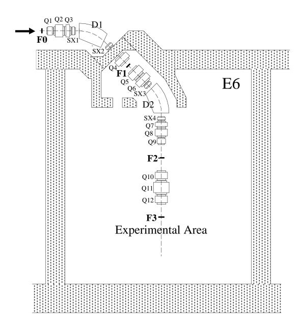
Figure 3.2: Layout of the radioactive beam line RIPS. The separation of the secondary beam is achieved in two stages: F0-F1 and F1-F2. The F3 focus was used to locate the secondary target.
