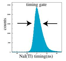
Figure A.3: Time spectrum of NaI(Tl) scintillators detectors. The  $\gamma$ -rays from the reaction products are selected by the gates indicated by the Gaussian component. The constant component was due to the background components.
