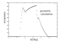
Figure 4.19: Detector acceptance of the SSD as a function of the angle in the laboratory flame. The data is obtained from the geometrical calculation.
