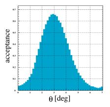
Figure 4.22: Detector acceptance of the SSD as a function of the angle in the laboratory flame from the Monte Carlo simulation. The finite size and angular spread of the incident beam is take into accounted in the data.
