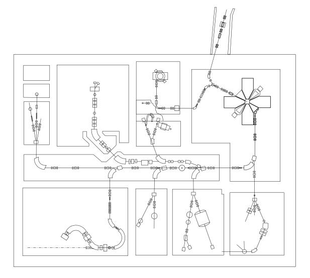
Figure 3.1: Layout of the RIKEN Accelerator Research Facility (RARF). An  $^{40}$ Ar beam was pre-accelerated with the AVF Cyclotron and was mainly accelerated up to 95 MeV/nucleon with the Ring Cyclotron. The beam is transported through the beam transport line in the room D onto the production target at RIPS. The fragment separator RIPS [13] lies in the room D and E6.
