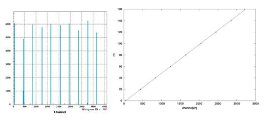
Figure 4.1: Plot of channel versus timing in ns. This calibration was fitted by a linear function of the timing.
