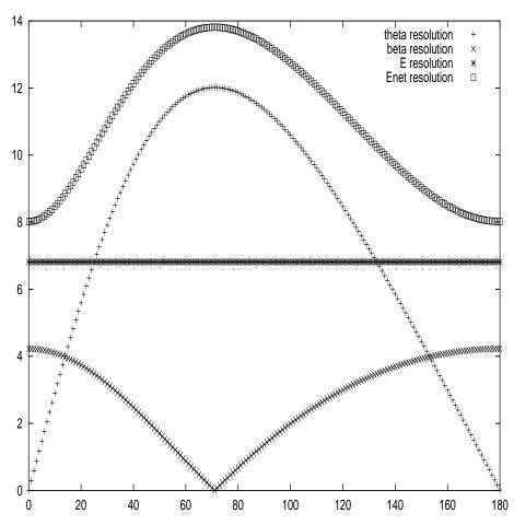
Figure A.11: Energy resolutions for 2 MeV  $\gamma$ -ray emitted from moving sources with v/c $\approx$ 0.32. Enet is the energy resolution of the Doppler corrected spectrum.
