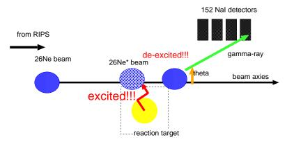
Figure A.4: Schematic view of in-beam  $\gamma$  spectroscopy. The theta is the  $\gamma$ -ray detection angle with respect to the beam axis in the laboratory frame.
