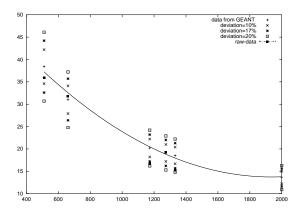
Figure B.3: Plot of photo-peak efficiencies as a function of  $\gamma$ -ray energies. The values measured by using  $\gamma$ -rays standard sources are plotted. The solid line represents the calculated values by **GEANT** code, which reproduces well measured efficiencies.
