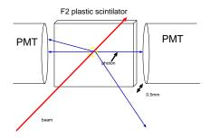
Figure 3.4: Schematic view of the F2 plastic scintillator.
