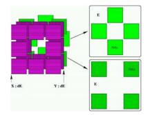
Figure 3.7: The Schematic view of SSD. Left:particle identification of the fragments was performed by using four-layer Si strip detectors (SSD) composed of  $\Delta E$  and E counters located at about 1.2 m downstream of the target.
