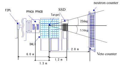
Figure 3.6: Schematic view of the setup backward F3.
