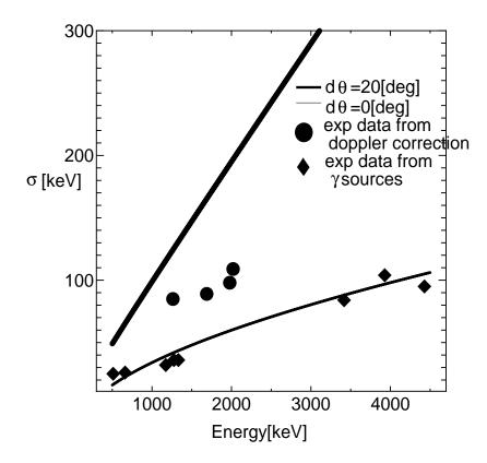
Figure A.10: Energy resolution function of  $\gamma\text{-ray}$  energy emitted from moving sources .
