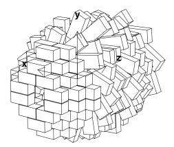
Figure 3.9: Schematic view of 152 NaI(T) scintillation detectors (DALI2).
